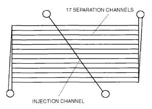
The device consists of mainly 50 x 10  $\mu$ m capillaries. The parallel channels are located at distances of 500  $\mu$ m. The introduction channel is placed at an angle to obtain identical distances between the electrodes at the ends of the parallel channels.
